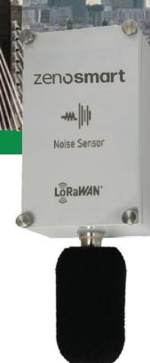
Operates with a 3.6V 19A battery and transmits data via LoRaWAN Gateway. The data transmission interval is adjustable, with monitoring and reporting available through [zenosmart.com](https://zenosmart.com). The sensor helps create quiet environments in cities and ensures safe working conditions in workplaces.
