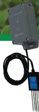
ZenoSmart operates with the LoRaWAN Gateway simply by connecting the cables. It can be configured via the IoT interface, and the data transmission frequency can be adjusted. Monitoring and reporting can be done through ZenoSmart.com. Large areas can be managed using LTE or Wi-Fi Gateways, and connection to the Helium network is possible. Soil EC and moisture sensors enable water savings and efficient agricultural management.
