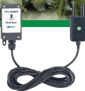
Insert the battery and place the probe into the soil to enable data transmission via the LoRaWAN Gateway. Data can be monitored from the IoT server, and the transmission frequency can be adjusted. With low power consumption, agricultural fields and soil moisture can be efficiently managed. The module helps optimize fertilizer usage with accurate pH measurements, preventing economic losses and environmental pollution.
