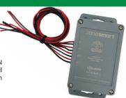
The irrigation module automatically irrigates by measuring soil temperature and moisture. LoRa and Bluetooth provide remote control and configuration. A soil sensor and water meter enable efficient irrigation and water consumption monitoring.
